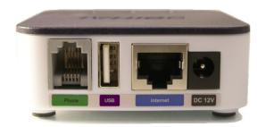
The OBi200 is a dedicated device, built with a high-performance system-on-a-chip platform to ensure high quality voice conversations. The OBi200 has high availability and reliability because it is always-on to make or receive a call. With the OBi200, a computer is not required and a computer does not need to be on to talk to people. To get started, all you need is a phone, power and a connection to the Internet.
