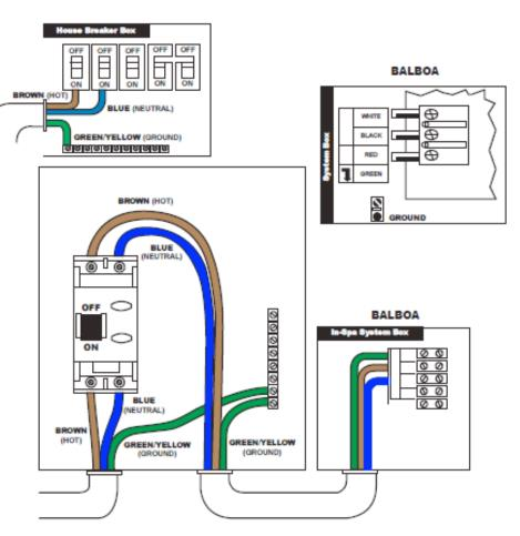
32 AMP GFCI WITH A-RATED TRIPPING CURRENT NOT EXCEEDING 30 MA.
