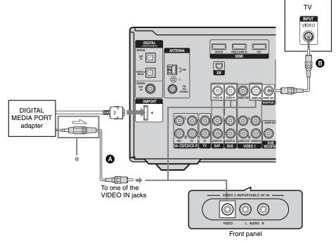
\* The type of connector varies depending on the DIGITAL MEDIA PORT adapter. For details, see the operating instructions supplied with the DIGITAL MEDIA PORT adapter.
