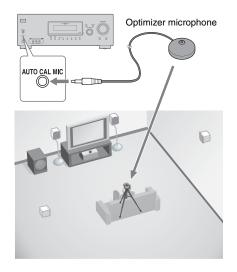
1 Connect the supplied optimizer microphone to the AUTO CAL MIC jack on the front panel.
