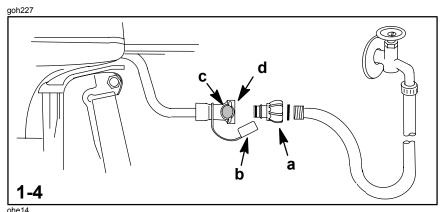
Flushing The Cooling System – Models with Hose Flush Attachment
