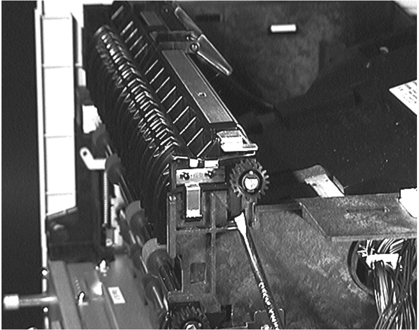
Figure 6-55 Upper Delivery Assembly Tabs
