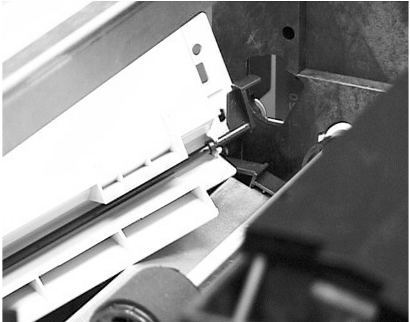
Figure 6-16 Tray 1 Inner Cover Flag (view from inside printer, left side)
