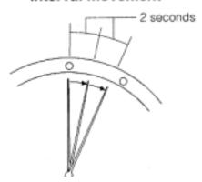
The second hand moves at two-second intervals to indicate that the watch is insufficiently charged. Although the watch will continue to operate normally at this time as well, it will stop after about 2 days have elapsed since the start of two-second-interval movement. Expose the watch to light to return the second hand to one-second interval movement.
