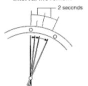
When the watch is again exposed to light after stopping, although the second hand begins to move, since the time is incorrect, the second hand moves irregularly at two-second intervals to indicate that the time is incorrect. Reset the time after the watch has been sufficiently charged. The second hand will continue to move irregularly at two-second intervals unless the time is reset.
