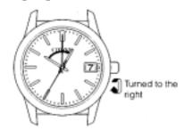
Direction of improper time difference correction
