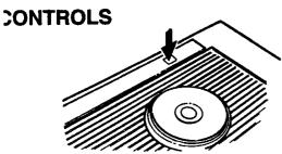
urn the downdraft blower ON by pressing down on the activating witch. The air vent will rise.
