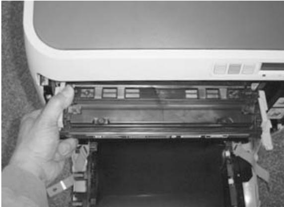
Installing the cartridge at an angle can damage or break the E-label reader guide pin.
