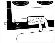
**NOTE:** The unit will not work if the control panel is not properly mounted. Plug the unit back in, turn on and continue use. If the unit still does not operate, repeat the steps above or call a Waring Certified Customer Service Center for assistance.
