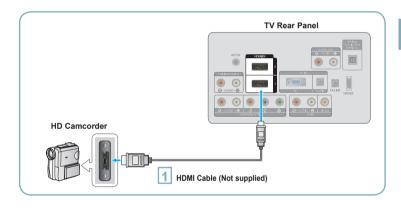
Connect an HDMI Cable between the HDMI IN (1 or 2) IN jack on the TV and the HDMI OUT jack on the camcorder.
