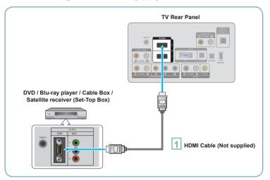
Connect an HDMI Cable between the HDMI IN (1 or 2) jack on the TV and the HDMI jack on the DVD Player or Cable Box / Satellite receiver (Set-Top Box).
