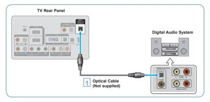
Connect an Optical Cable between the DIGITAL AUDIO OUT (OPTICAL) jacks on the TV and the Digital Audio Input jacks on the Digital Audio System.
