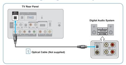
Connect an Optical Cable between the DIGITAL AUDIO OUT (OPTICAL) jacks on the TV and the Digital Audio Input jacks on the Digital Audio System.
