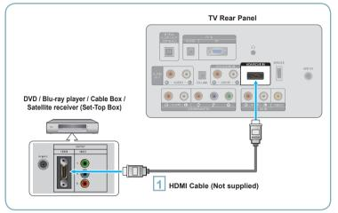
Connect an HDMI Cable between the HDMI (DVI) IN jack on the TV and the HDMI jack on the DVD / Blu-ray Player or Cable Box / Satellite receiver (Set-Top Box).
