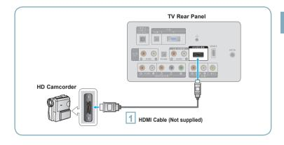
Connect an HDMI Cable between the HDMI (DVI) IN jack on the TV and the HDMI OUT jack on the camcorder.
