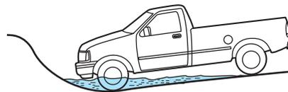
Once through water, always try the brakes. Wet brakes do not stop the vehicle as effectively as dry brakes. You can dry the brakes faster by driving the vehicle slowly while applying light pressure on the brake pedal.
